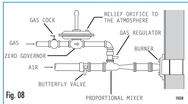
ments, we recommend pressure  $P_1$ ,  $P_2$  and  $P_3$  be controlled. It is possible to verify whether the mixer works correctly by comparing the data obtained to what we have described above. If after some time some anomalies are detected, it is advisable to check the 3 pressures: this is the quickest and easiest way to find out the cause of the anomaly.
