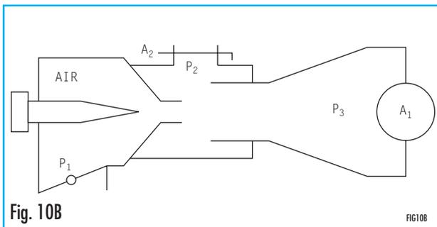
Figure 10B shows a mixer with a needle regulator placed in order to adjust the area of the air injector. In proportional mixers it is not possible to obtain satisfactory working conditions if at any change in section  $A_1$  does not correspond a proportional change in the area downstream of the injector. Theoretically there exists only one ideal ratio between the area of injector  $A_1$  and the area  $A_T$  of the mixer throat.
