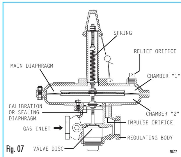
Should we apply a positive or negative pressure in this chamber, downstream of the valve a pressure would result which would be exactly the same as the pressure applied to the upper part of the main diaphragm. That is why the relief orifice of chamber (1) must never be connected via any exhaust pipe to the chimney, as is the case with standard pressure reducing valves.
