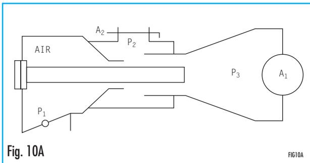
Figure 10A shows a mixer where the regulation of this area is done by replacing a cylindrical section adjuster. When some cylinders featuring different diameters are placed in the venturi throat, different capacities are obtained. In this case, the air injector is an annular injector.
