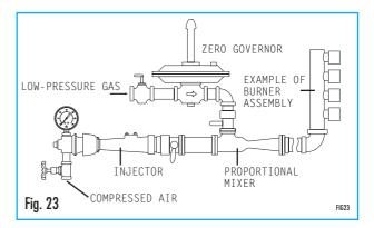
the proportional mixer, as the total pressure of the mixture may be easily controlled by means of the needle valve of the compressed air injector (Fig. 23).
